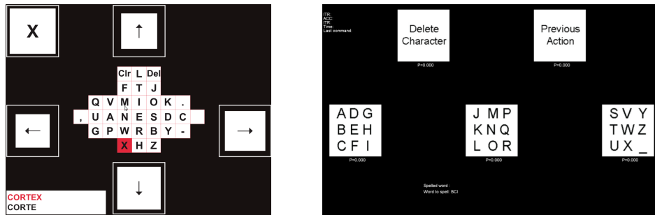
Figure 3.4: Variants of SSVEP interfaces. Left: Bremen-BCI (refer to [Vol11]). Right: The calibration-free CBCI (refer to [Cec10a])
