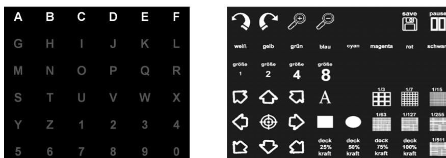
Figure 3.3: Variants of P300 input matrices based on BCI2000. Left: P300 standard matrix. Right: P300 brainpainting matrix by [JSS + 10].
