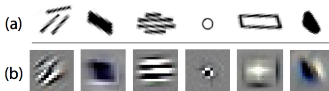
Figure 4.1: Representations in the third layer of a deconvolutional network in comparison to Marr's Place tokens. a) Place tokens from Fig. 2-4 of Vision by David Marr. b) 3rd-level representations from [Zeiler et al., 2010] (also the illustration source).
